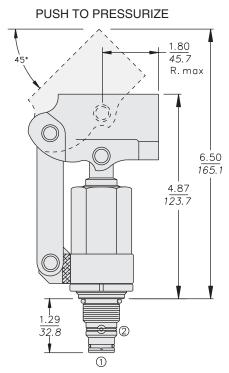
The Beam (Handle Socket) Inside Diameter 0.85" (21.6 mm) Beam Rotates around Vertical Axis for 360 Handle Positioning
