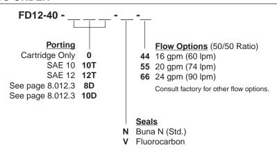
NOTE: Standard 12-size 4-way bodies should not be used for flow dividers. See special flow divider bodies, page 8.012.1
