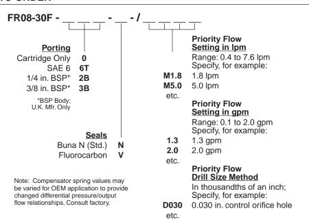
Note: Minimum drill diameter is 0.020 in. For smaller orifice sizes consult factory.
