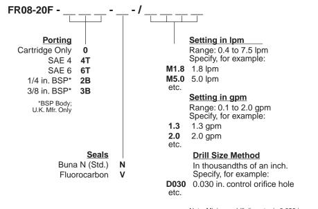
Note: Compensator spring values may be varied for OEM application to provide changed differential pressure/output flow relationships. Consult factory. Note: Minimum drill diameter is 0.020 in. For smaller orifice sizes consult factory.
