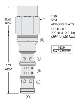
ORIFICE DISC CANNOT BE USED WITH THIS PRODUCT due to HyPerformance™ Cavity.
