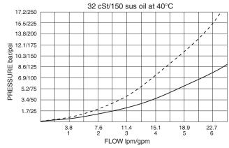
Performance with 12 VDC Coils and 10.3 bar/150 psi inline compensator (for other voltages consult factory)
