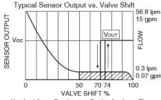
Hatched Area: Overlapping Stroke, Leakage Flow
