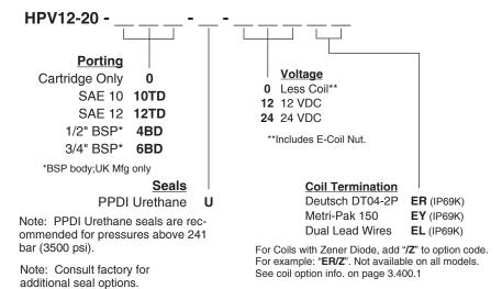
**Cartridge:** Weight: 0.29 kg. (0.64 lbs.) Steel with hardened work surfaces. Zinc-plated exposed surfaces. PPDI Urethane seals without back-up rings standard.
